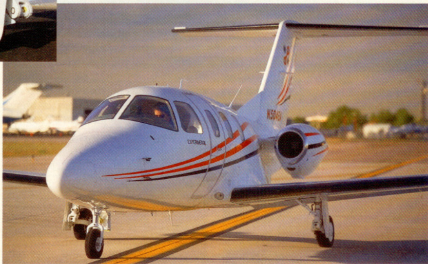
Combined with piston-single-type approach speeds, the trailing-link main landing gear promises a smooth arrival.
