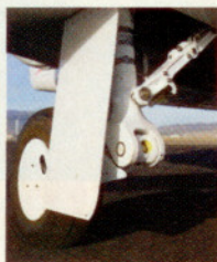
Combined with piston-single-type approach speeds, the trailing-link main landing gear promises a smooth arrival.
